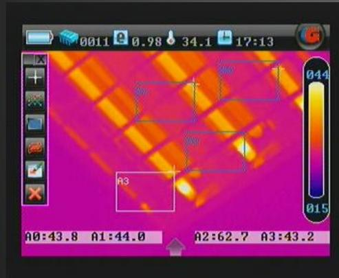
Ø Auto hot-spot tracing and center-cursor temperature display
